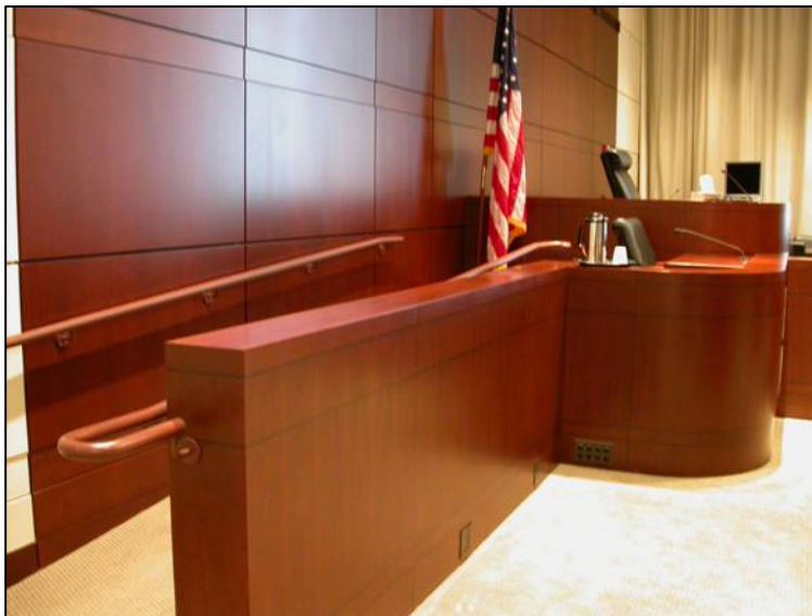
Figure: Ramp access to witness stand.
