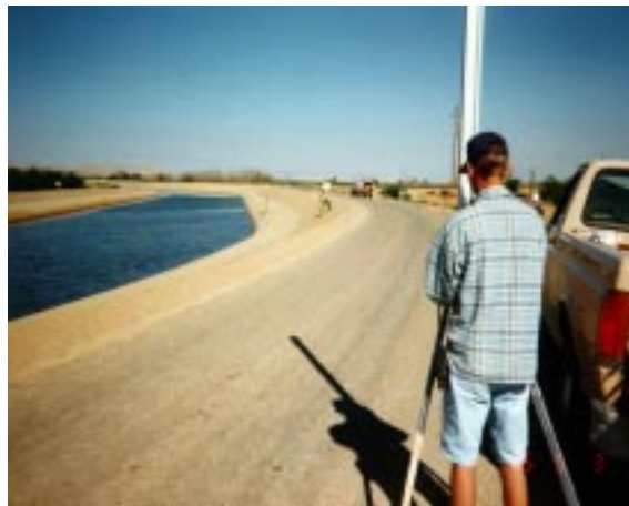
Figure 14 Subsidence Monitoring Along an Irrigation Channel
