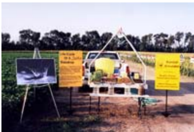
small portable rainfall simulator first built in Kansas by district conservationist Clyde Mermis and the Lawrence Field Office NRCS staff (NRCS photo -- click to enlarge)
