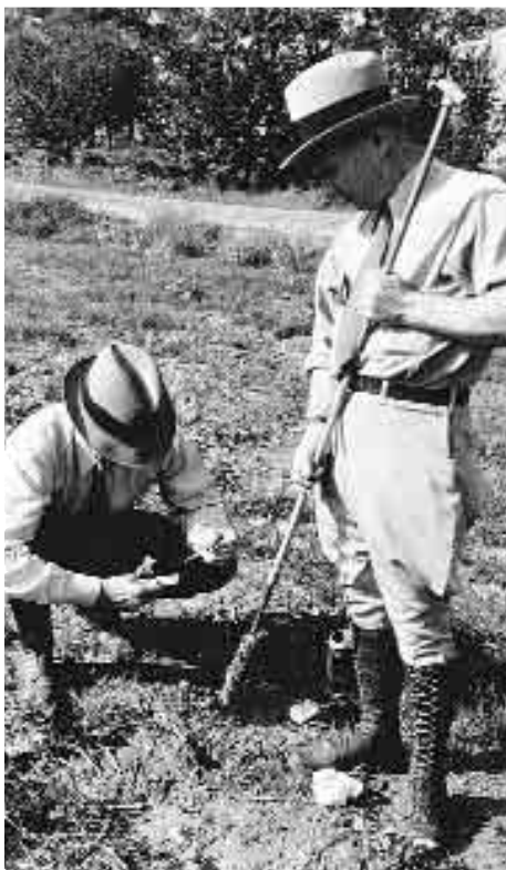
The screw auger was the primary tool used by the soil scientist in the early days. Texturing by hand was one of the first "soil tests" and continues to be a tool for the soil scientist today.
