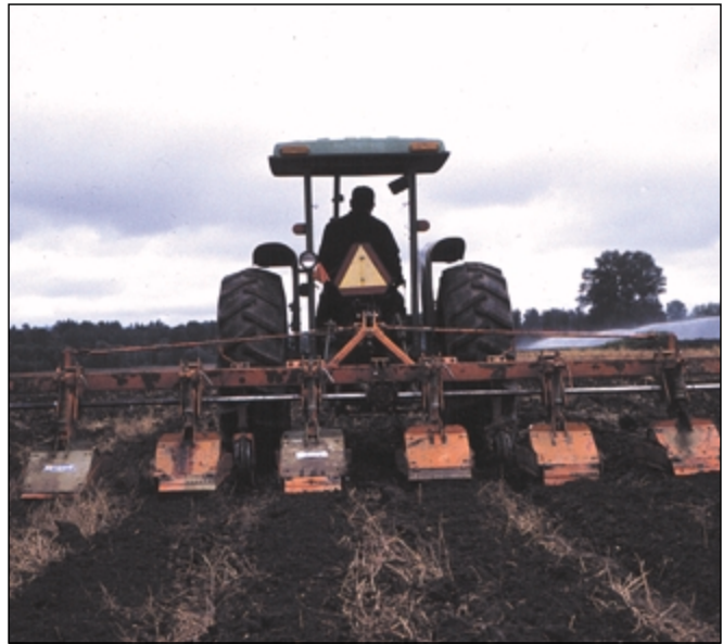
Figure 8.—A light-duty rotary cultivator can be used for a second-pass tillage pass in strip-till systems to improve seedbed quality.
