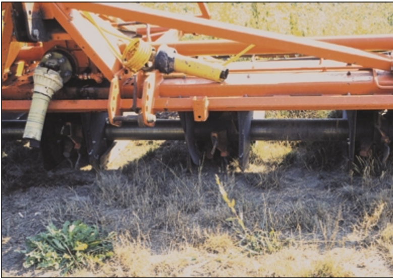
Figure 10.—The Howard Rotospike tiller shown here has been modified with soil shields for use in second-pass operations in strip-till systems. The closeup view on the right shows the heavy-duty spikes, which are used instead of traditional L-shaped tines.
