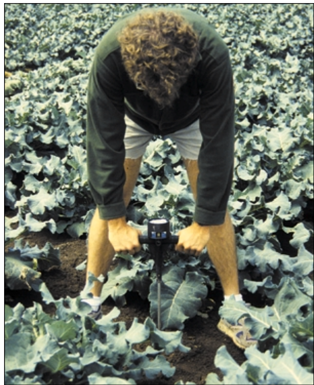
Figure 12.—The DICKEY-john penetrometer is a useful tool for testing soil compaction at varying soil depths.
