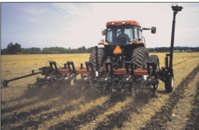
Figure 7.—The Unverferth Ripper-Stripper strip-till machine is similar to the Transtiller, using a subsoiling shank and pairs of fluted coulters to prepare a seedbed.
