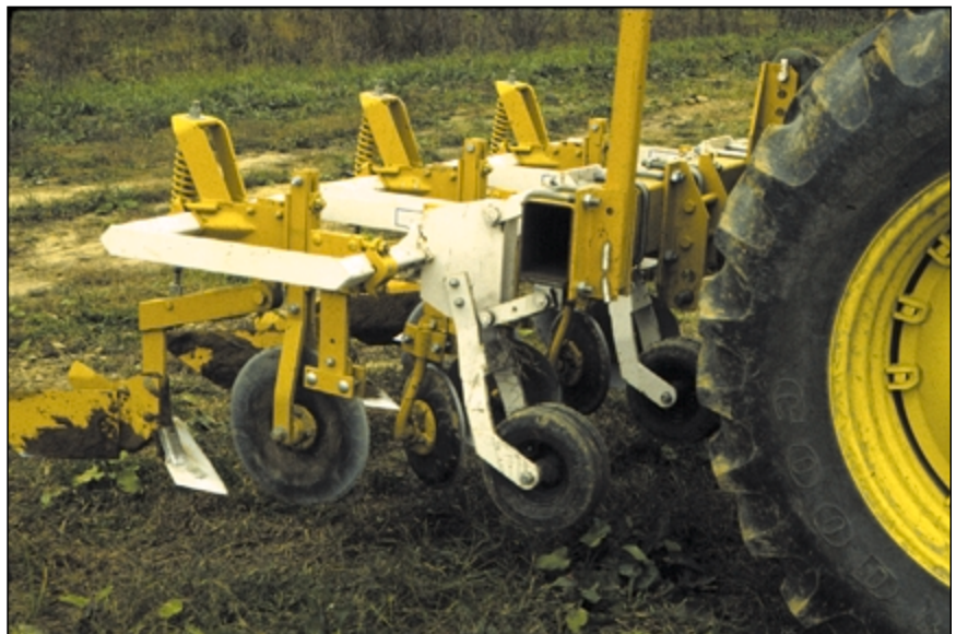
Figure 14.—Components of the Buffalo cultivator that allow it to operate in high-residue conditions include a rolling disk coulters to cut through residue in front of the heavy-duty sweep cultivators.
