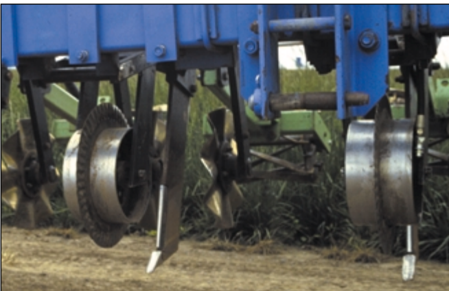
Figure 6.—Closeup view of the Transtiller strip-till machine, showing the front disk coupler with depth gage band, followed by the tilling shank, fluted coulters, and finishing basket.
