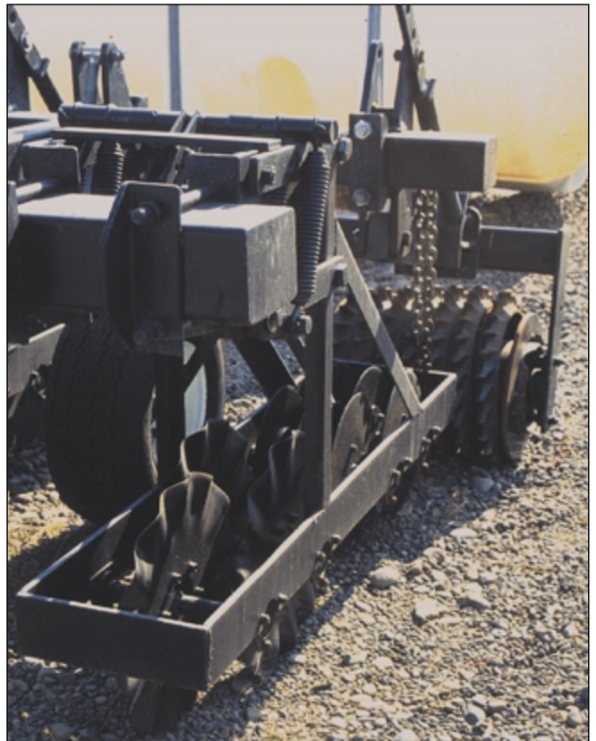
Figure 9.—One approach to second-pass equipment for strip-till is this machine, which uses a series of flat disks followed by a ring roller (designed by J. Hendricks and R. Heater).
