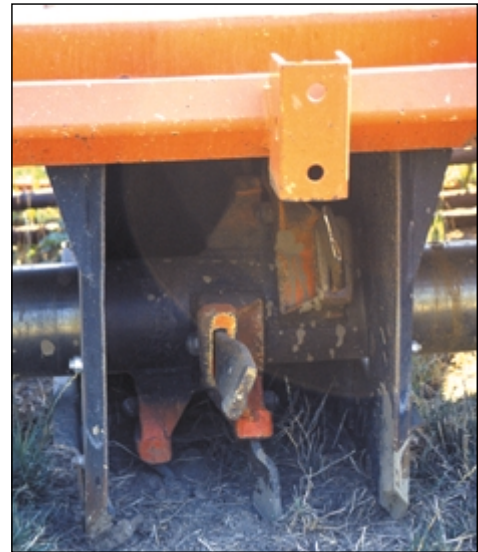
Figure 10.—The Howard Rotospike tiller shown here has been modified with soil shields for use in second-pass operations in strip-till systems. The closeup view on the right shows the heavy-duty spikes, which are used instead of traditional L-shaped tines.
