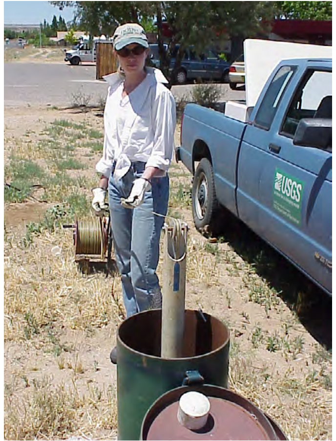
A USGS hydrologist measuring ground-water levels with an electric tape in a monitoring well in Albuquerque, New Mexico (photograph by James R. Bartolino, U.S. Geological Survey). Frequent and consistent measurements of ground-water levels are crucial for understanding the aquifer system and tracking water-level declines.
