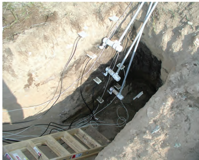
Unsaturated-zone instruments used to estimate ground-water recharge are installed in oil-saturated soils at the Bemidji, Minnesota, research site.
