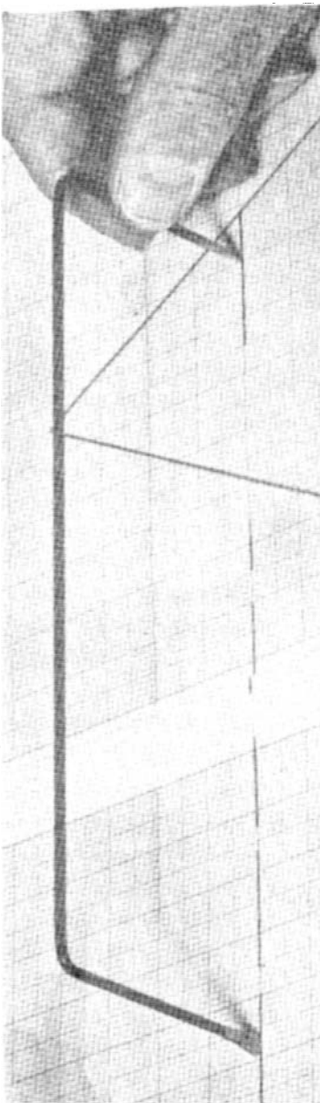
Figure 20. Homemade hatchet planimeter is calibrated by measuring regular figures of known areas.
