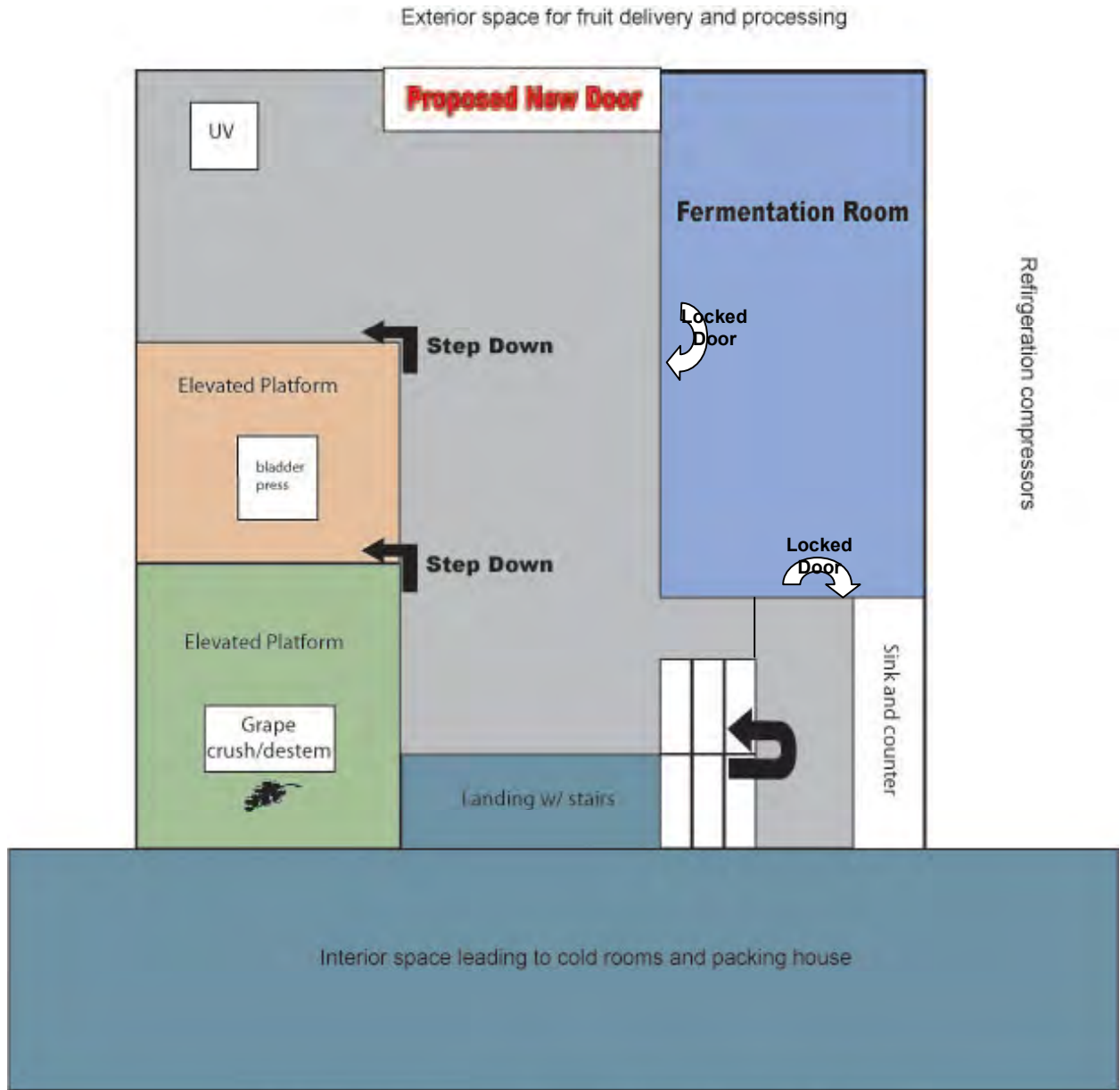
Cider/Juice/Winery Facility Layout at UMass Cold Spring Orchard Research and Education Center Belchertown, MA
