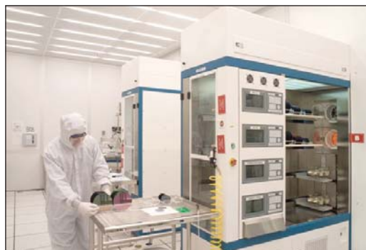
Figure 2. Oxidation and annealing furnaces banks.
