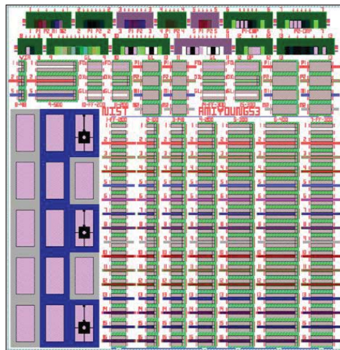
Figure 1. CMOS test chip design incorporating thickness test structures, cantilevers, fixed-fixed beams, and tensile test structures.
