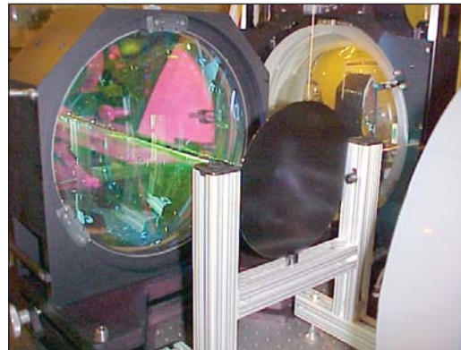
Figure 1b. Test end of the IR^2 setup for TTV measurements of 300 mm wafers. The picture shows the collimator lens together with a silicon wafer and a return flat.
