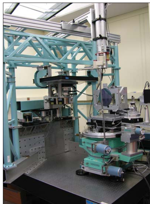
Figure 3. Ceramics Division Parallel Beam Diffractometer (CDPBD). Showing a rotating anode X-ray source (center left), monochromator for generating parallel/monochromatic X-rays (upper center), angle-encoded rotation stages for measuring diffraction angles (lower right) and receiving optics/detector (center right). In order to achieve accuracy in angle measurements and X-ray wavelength stability, numerous design features of varying complexity are present ranging from a "floating" platform holding the X-ray source to a hanging second rotation stage (top center) designed specifically to rotate the cables for the diffraction rotation stages.
