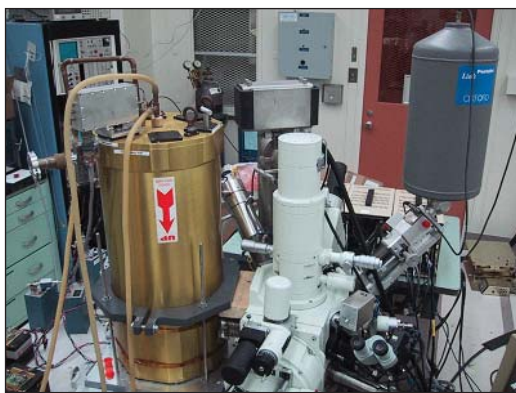
Figure 1. Single-pixel NIST X-ray microcalorimeter system on a scanning-electron microscope. The system was developed in the Electronics and Electrical Engineering Laboratory (EEEL) at NIST, Boulder, and transferred to the Chemical Science and Technology Laboratory (CSTL) at NIST Gaithersburg to be used to study problems of interest to the semiconductor industry.
