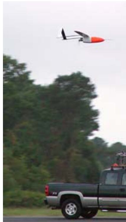
Aerosonde release from its transport vehicle on the runway at the NASA Wallops flight Facility
