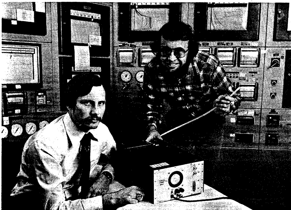
Fig. 42. Alan Hawthorne and Dick Gammage in 1981 with a derivative ultraviolet absorption spectrometer that was designed for the analysis of sulfur dioxide and low boiling point aromatics.
