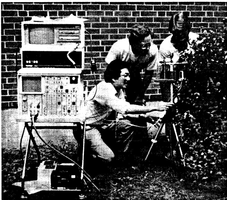
Fig. 52. Field testing of a fiber-optic microprobe instrument by Tuan Vo-Dinh, Gordon Miller, and Michelle Dial (left to right). This instrument was developed to assess the effects on terrestrial plant life of increased levels of ultraviolet radiation due to ozone depletion in the atmosphere.
