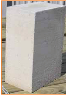
Commercial-scale, autoclaved aerated concrete blocks made using Class C fly ash from the Baldwin power plant.
