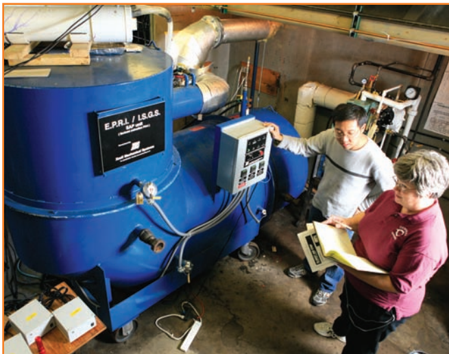
Xu Chen and Kathy Henry at the ISGS Applied Research Lab with the transportable bench sorbent activation process (SAP) unit, a patented technology developed at the ISGS.
