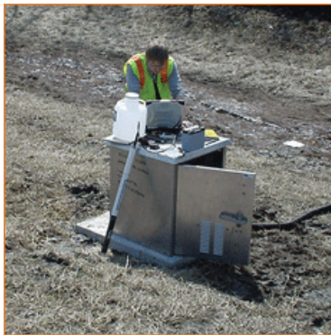
Charles Knight, ISGS scientist in the Wetlands Section, collects discharge data from a roadside ditch at the future site of a bioswale along I-294 in Des Plaines, Illinois.
