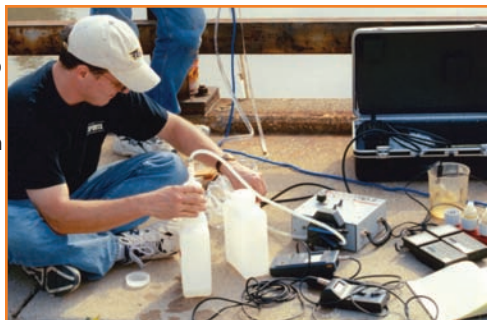
Filtering water samples for isotopes of nitrates.
