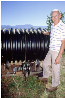
In Sequim on Washington's Olympic Peninsula, Jack Caldicott has created a labor-saving compost turner.
