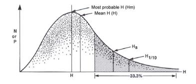
Also shown are the mean wave height (H), most probable wave height (Hm), and the height of the highest 10% of waves (H1/10). The mean wave height H is approximately equal to 2/3rds (0.64) the value of Hs and H1/10 is approximately equal to 1.27 times the value of Hs. In addition, the height of the highest 1% of waves (H1/100) is approximately equal to 1.67 times Hs, and a theoretical maximum wave height (Hmax) is approximately equal to *two times Hs*.
