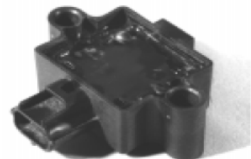
Example of anti-lock braking sensor from a 1999 Jeep Grand Cherokee. Photo credit: Jeff Gearhart
