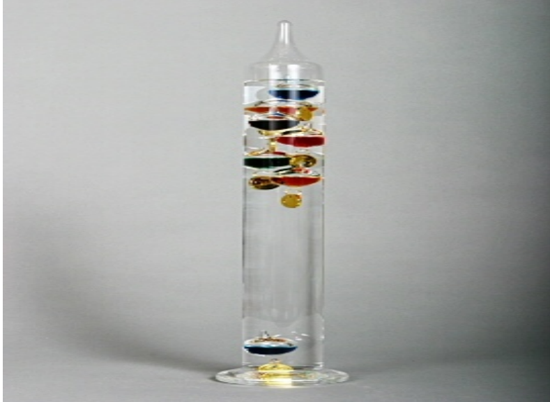
Galileo Thermometer: contains spheres in a liquid. The current temperature is indicated by the lowest floating glass sphere in the cylinder.
