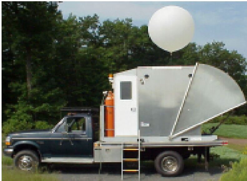
Radiosonde: contains instruments which measure air temperature, humidity, and pressure with height, to heights less than 30 Km.
