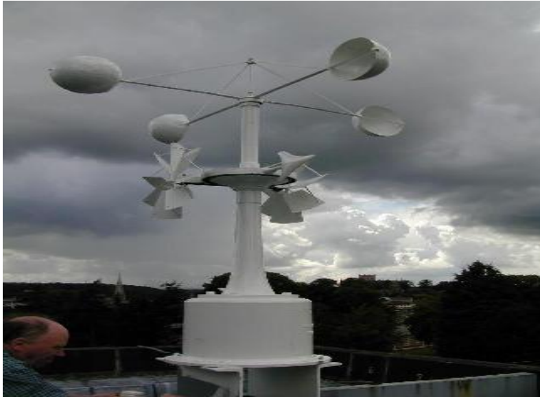
Anemometer: measures the velocity or speed of the wind.
