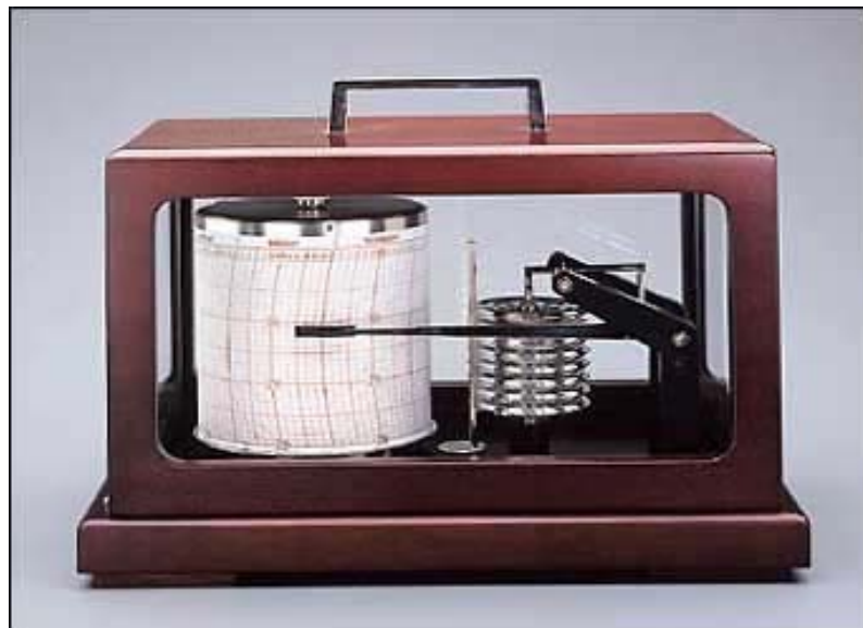
Barograph: automatically records changes in air pressure.
