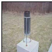
Rain gage or Rain gauge: uses for measuring rainfall; an instrument is large or small container size.
