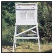
Instrument shelter: protects temperature and relative humidity sensors and other instruments against errors and damage due to solar radiation, wind, and precipitation.
