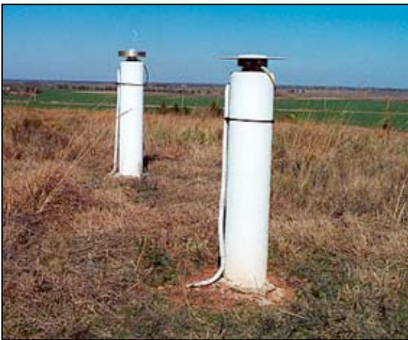
GPS receivers are installed at all the extended facilities throughout the SGP domain (ARM photo).
