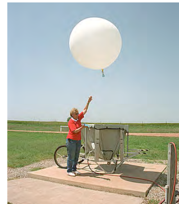
A technician releases a white balloon-borne sounding system at the Southern Great Plains site. Courtesy: U.S. Department of Energy's Atmospheric Radiation Measurement Program.
