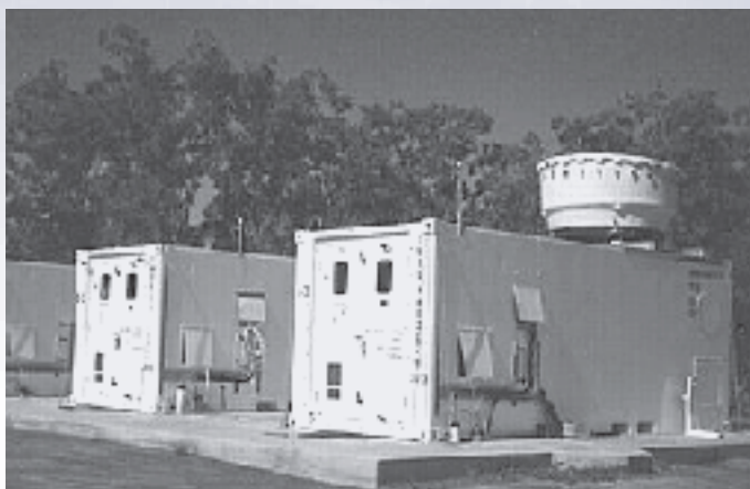
An instrument shelter houses the MMCR; the large object on top of the shelter is the MMCR antenna.
