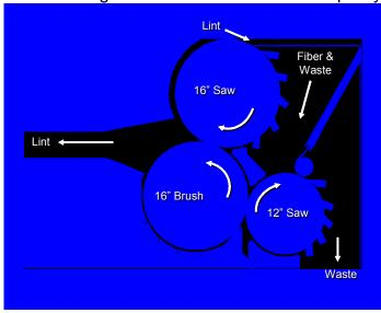
cleaner operated for a full ginning season at a commercial gin without operational problems. Measured HVI and AFIS parameters of the baled lint from the experimental lint cleaner generally equaled or exceeded those of the standard lint cleaner. This technology would benefit cotton producers and ginners by reducing filer wastes from conventional saw-type lint cleaners.
