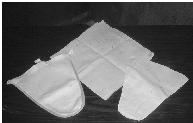
Figure 4. Maple syrup filters. From left to right, a cone filter designed to be suspended in a tank or large can, a square filter intended to be laid flat on a screen, and a prefilter intended to be placed inside a cone filter to extend its useful life.
