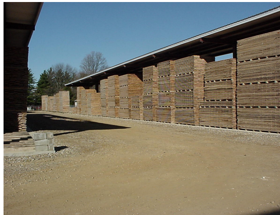
Figure 2. Air drying yard, Brenneman Lumber Co.
