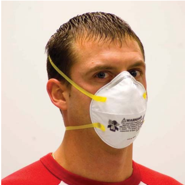
Figure 2. Properly donned disposable N95 filtering facepiece respirator. To be properly donned, the respirator must be correctly oriented on the face and held in position with both straps. The straps must be correctly placed, with the upper strap high on the head and the lower strap below the ears. For persons with long hair, the lower strap should be placed under (not over) the hair. The nose clip must be tightened to avoid gaps between the respirator and the skin. Facial hair should be removed before donning. Photo used with permission.
