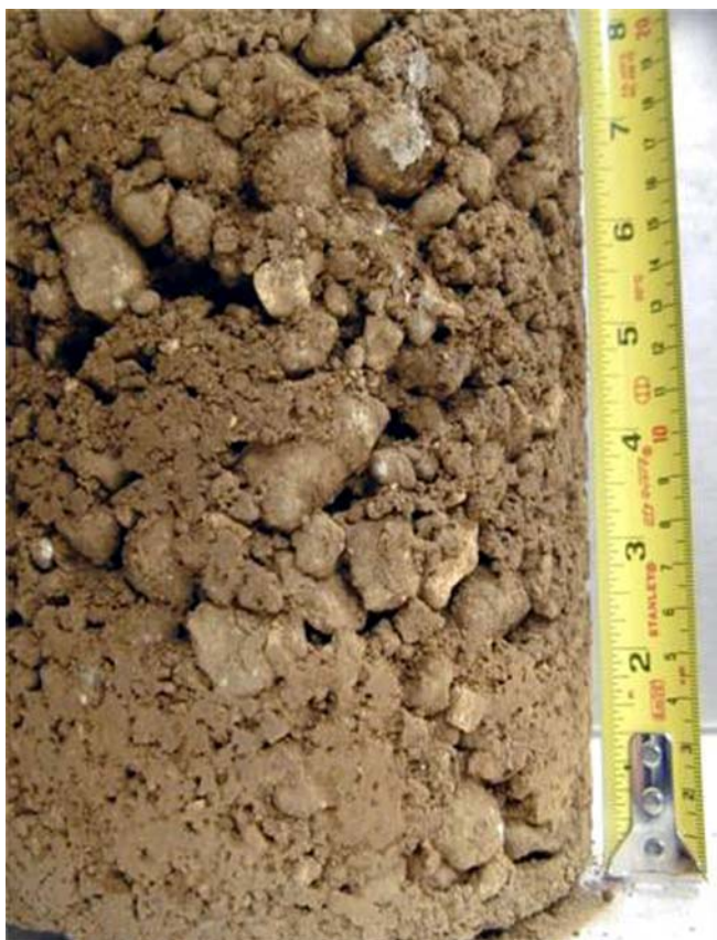
Figure 4. The profile of a gravelly soil. The soil is typical of soils found in the Homestead area, in the southern peninsula of Florida.
