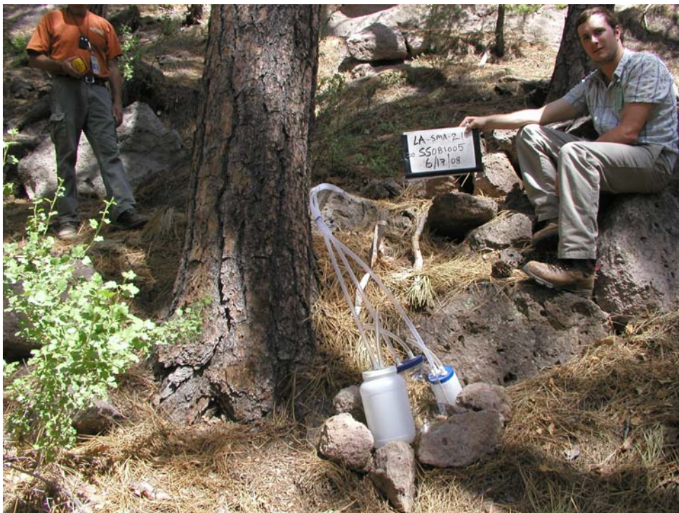
Figure 3.1-4 LA-SMA-2.1, the existing sampler at the outfall of SWMU 01-001(f)
