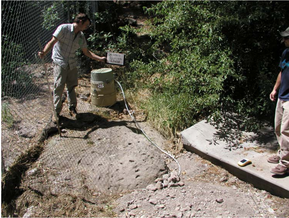
Figure 3.1-3 LA-SMA-2, the run-on sampler located at the upstream end of the tributary canyon and just upgradient of the SWMU
