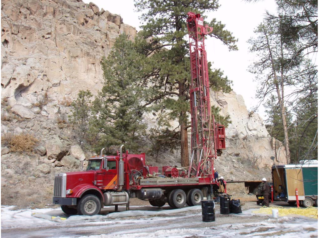
Figure 2.1-1 Atlas Topco TH60 rig used for retrieving Barcad sampling system from R-33
