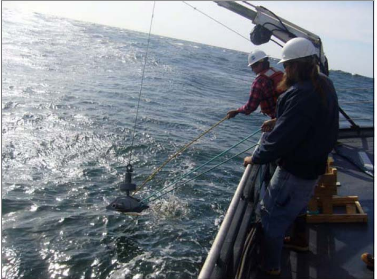
Figure 3.2: Shipek grab being deployed at MCR
