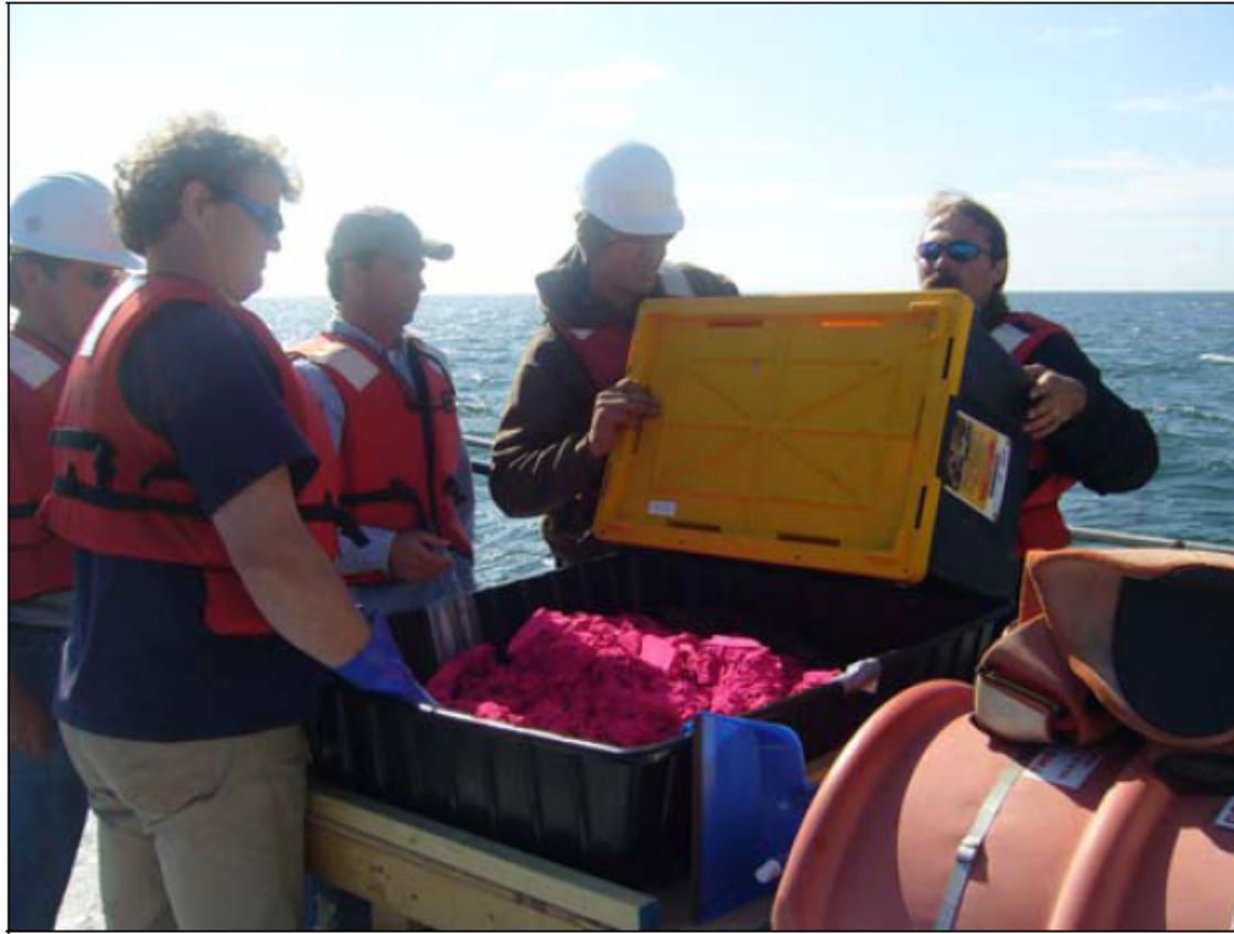
Figure 3.5: Tracer:sediment being transferred from the storage box into the hopper prior to being placed into the dissolving bags.
