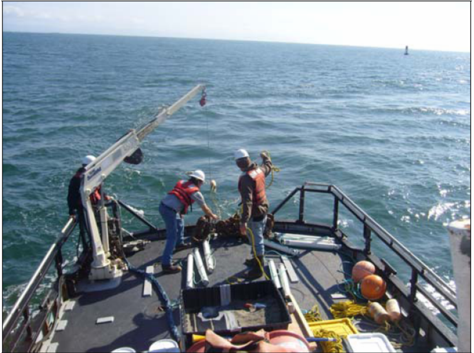
Figure 3.3: Deployment of the sediment traps, 1 October 2006
