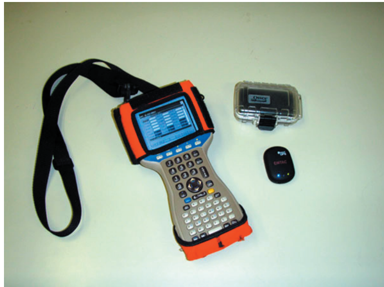
The Allegro data recorder and Bluetooth-enabled GPS device for electronic transmission of plot coordinates.
