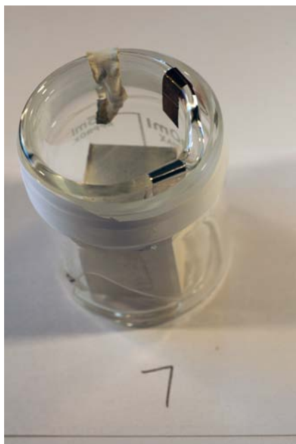
A small block of wood sample coated with sealant was inspected for off-gassing.
