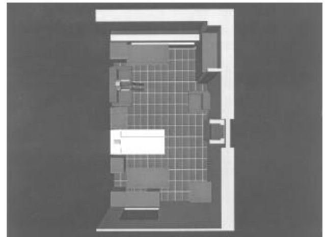
Figure 12 Plan view showing diffuser locations for low induction/low induction diffuser combination.
