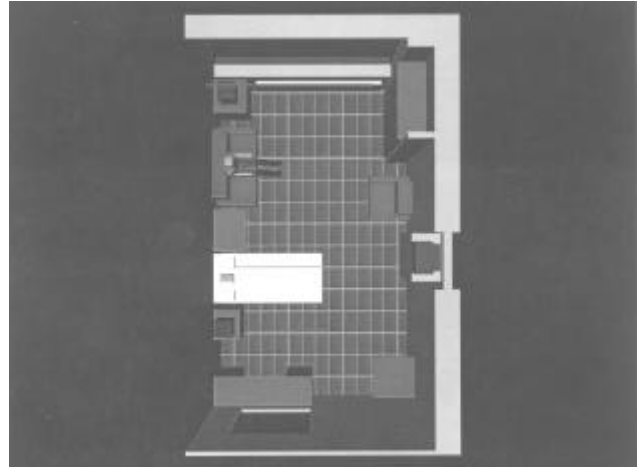
Figure 11 Plan view showing diffuser locations for linear/linear diffuser combination.
