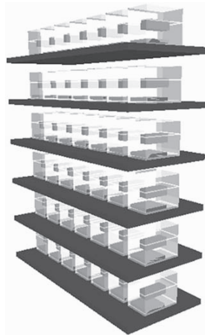
Figure 8 CFD model of cage rack.
