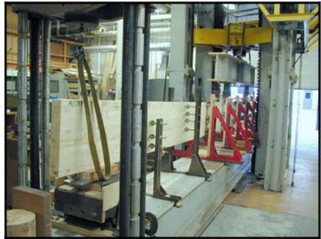
Researchers tested the properties of glulam beams made with mechanically graded ponderosa pine in hopes of providing a valuable use for the most common species in the western United States.
