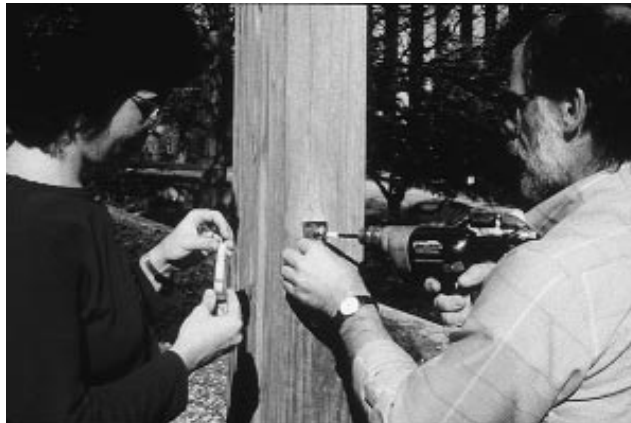
A test sample of wood shavings is removed by drilling a small hole.
