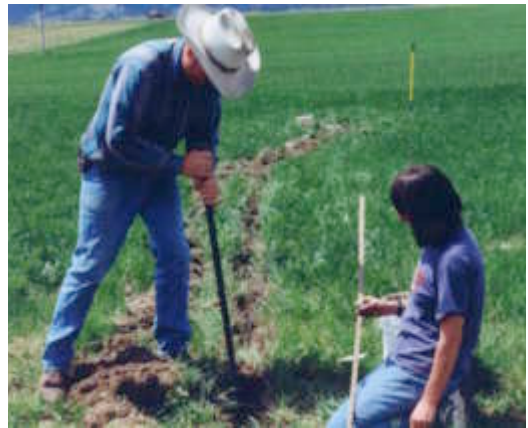
Using a bar to dig sensor holes. (NCAT photo)
