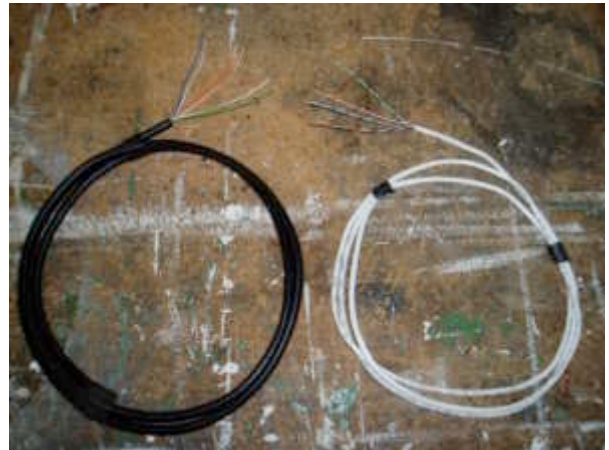
Direct burial cable and indoor phone wire. (NCAT photo)
