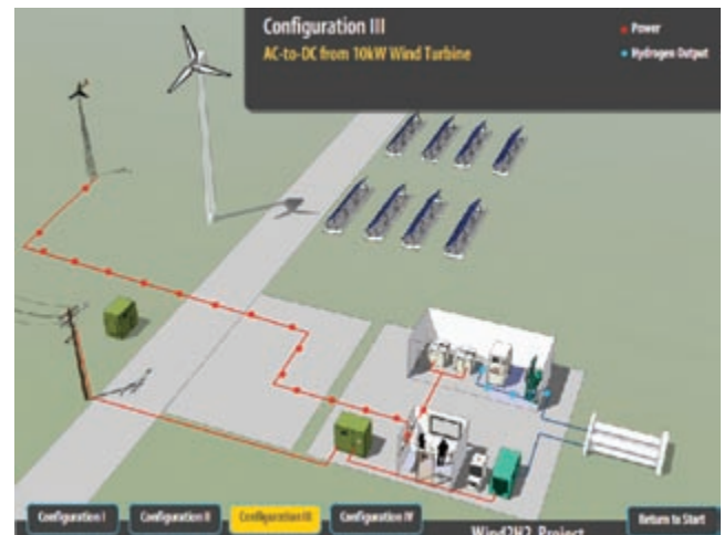
This wind-to-hydrogen animation at http://www.nrel.gov/hydrogen/proj_wind_hydrogen.html demonstrates how electricity from wind turbines is used to produce hydrogen at NREL's National Wind Technology Center.
