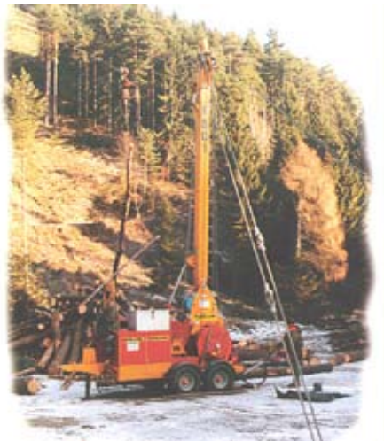
Figure 14. Towable skyline yarder. (photo courtesy of Koller)
