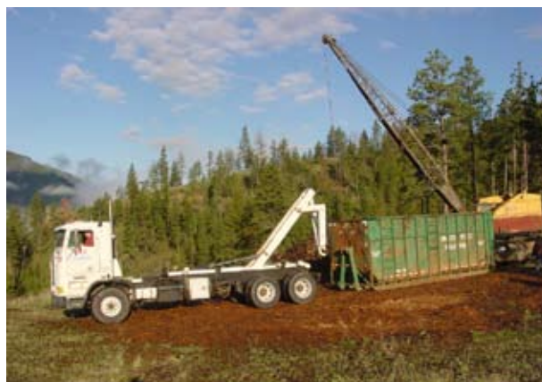
Figure 34—Roll-off container vehicle. Prototype stage, but transport vehicles like this may be economically feasible to use on low-standard roads when high ground clearance and maneuverable vehicles are required to gain access to biomass. (Photo courtesy of Craig Rawlings, Montana Community Development Corp. [MCDC])
