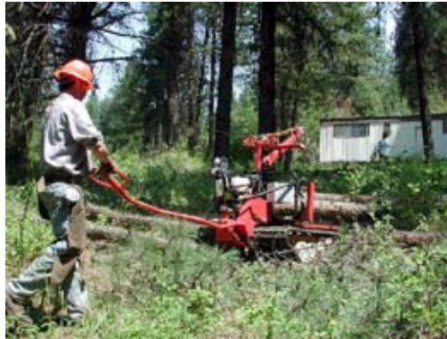
Figure 2—Iron Horse Pro mini-skidder.
