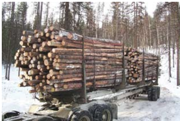
Figure 31—Short-log (18 foot) load of small-diameter sawlogs on double bunks. (Bonners Ferry Ranger District, Idaho.)
