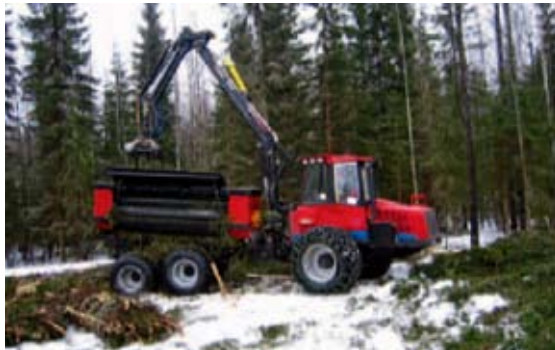
Figure 23—Another manufacturer's version of a slash bundling machine. This one quickly converts to a forwarder. (Photo courtesy of Valmet.)
