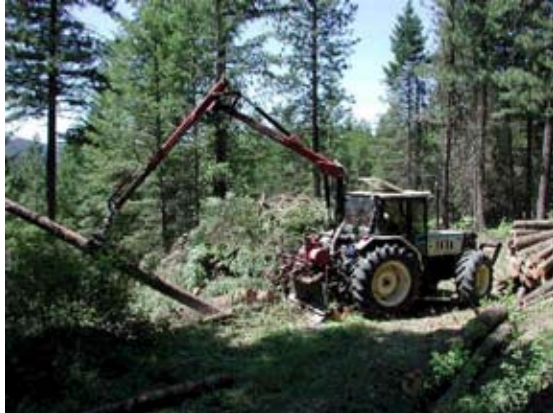
Figure 4—Modified farm tractor with log loader and remote-controlled winch.
