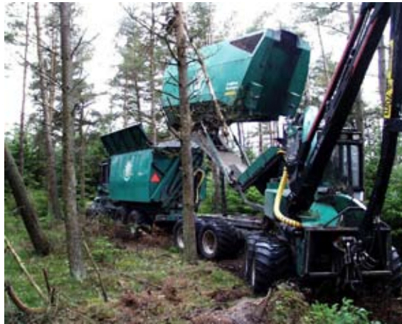
Figure 19—In-woods chipper and chip container transporter. (Photo courtesy of Karsten Frisk, Danish National Forest and Nature Agency.)
