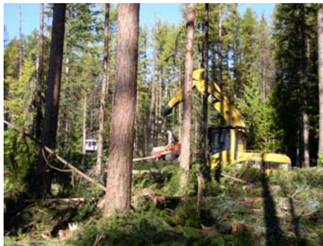
Figure 42—Same project area during fuels-reduction treatment. Pictured here is a feller-buncher in the background cutting trees and an in-the-woods processor in the foreground that is processing short logs down to a 4-inch top diameter. The logs are then skidded out using a grapple skidder.
