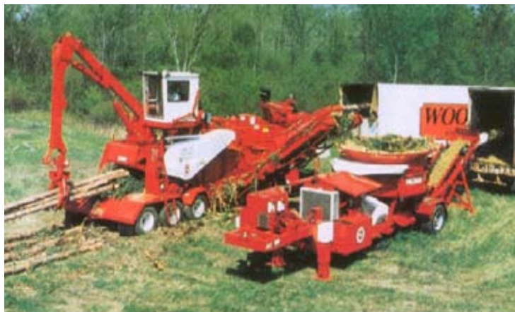
Figure 20—Dual chipping operation, flail chipper on left making “clean” pulp chips and tub grinder on right making “dirty” fuel chips. (Photo courtesy of Morbark, Inc.)
