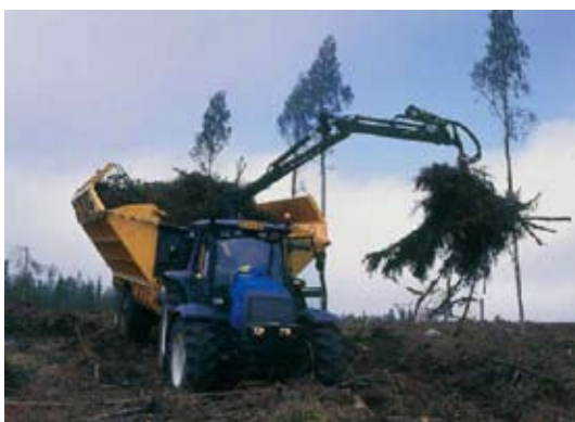
Figure 25—Load-compacting HavuHukka forwarder for transporting logging residues from stump to satellite terminals. (Photo courtesy of Vapo.)
