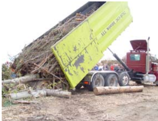
Figure 36—The roll-off container has a dumping feature and can be used to transport chips or loose slash. Economics would dictate short haul distances (Photo courtesy of Dave Atkins, USFS).
