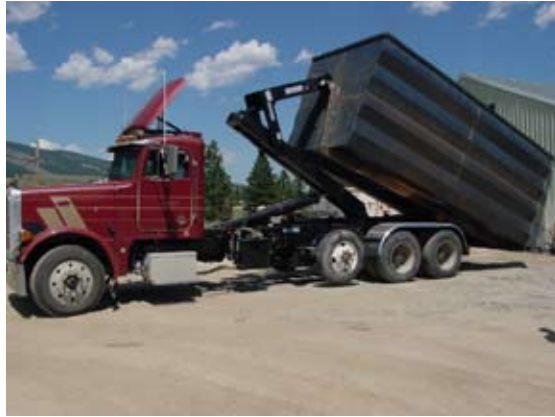
Figure 35—Another prototype version of a roll-off container vehicle. This one can transport two empty containers in a “nested” configuration. (Photo courtesy of Craig Rawlings, MCDC.)
