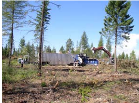
Figure 33—Standard chip van with a load capacity of about 30 green tons of chips. The vehicle is on a flat gravel road on private property being developed for residential construction. Notice low ground clearance and long length of chip van, which restricts its use on low standard forest roads. Slash piles are being chipped in a horizontal grinder and chips are being fed directly into van (Bonners Ferry, Idaho).
