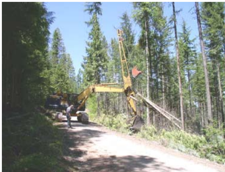
Figure 15. "Excaliner." (Excavator-mounted skyline yarder.)
