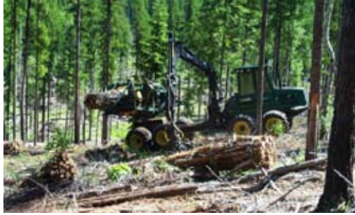
Figure 21—Timberjack 1490D Slash Bundler, first test site in North America, Bonners Ferry Ranger District, Idaho Panhandle National Forest (NF), 2003.
