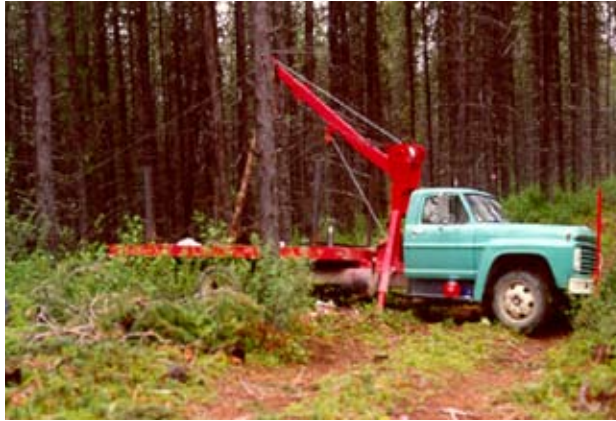
Figure 7—Home-built skyline-swing loader - hauler.
