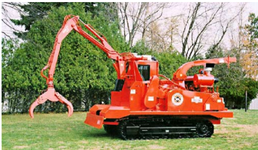
Figure 17—Morbark Model 20/36 Track Chipper. (Photo courtesy of Morbark, Inc.)
