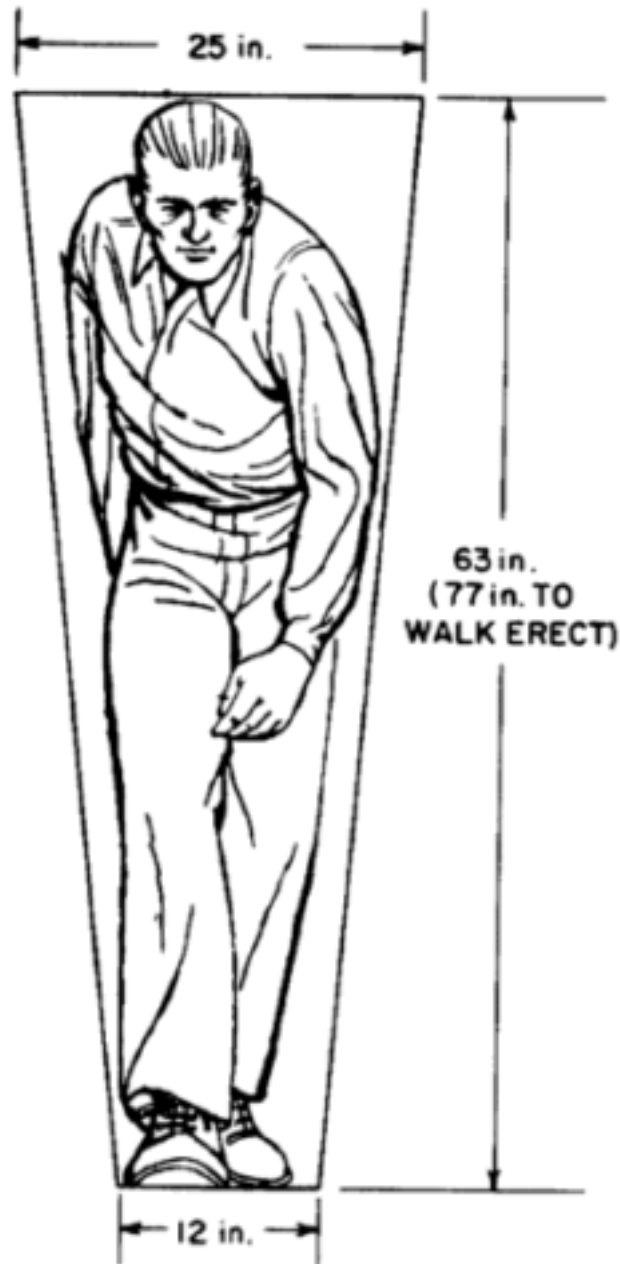
Figure 2 - Minimum catwalk widths. (2)
