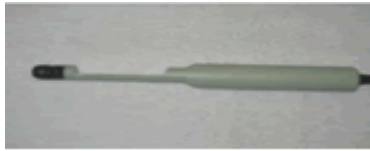
8808 Transducer (used for scanning and biopsy)
