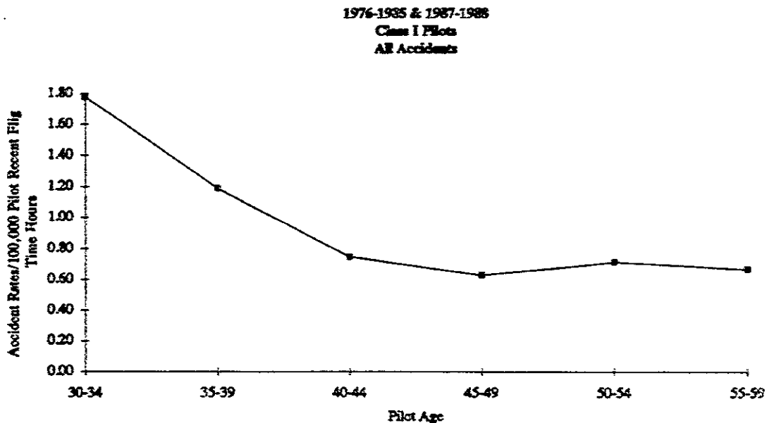
Figure 5-1. Accident rates for all Class I pilots for the years 1976-1985 and 1987-1988 as a function of age. Pilots were grouped in 5-year intervals. The numerator for rate was obtained by counting all accidents in the NTSB for the given group of pilots. The denominator was obtained by accumulating from the medical database the total annualized hours flown during the year by pilots in the given group. See Table 3-6 for the annualization factors.
