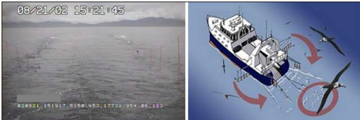
Figure 20. Left- example of streamer line imagery from an Alaska halibut longline vessel (Ames et al., 2005). Right- conceptual drawing of seabird streamer line device used to reduce seabird interactions with trawl warps (from Crysell, 2002).
