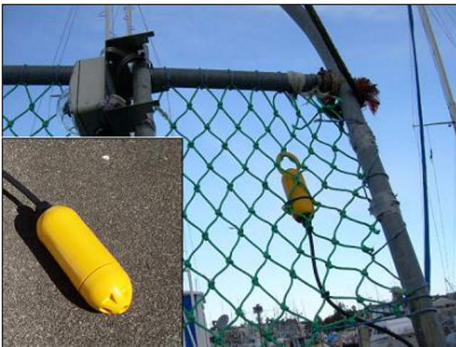
Figure A7. Hydrophone (inset) and shown mounted on the net cage.
