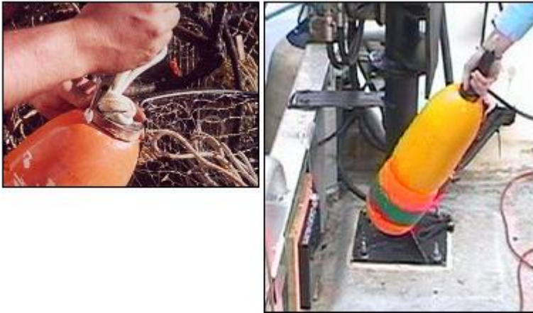
Figure A6. RFID chip inserted in crab buoy (left), and operation of scanning the buoy upon trap hauling (right).
