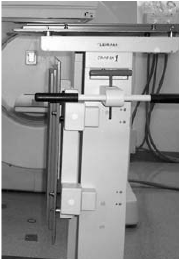
Figure 1-10. Collimators in Rack
