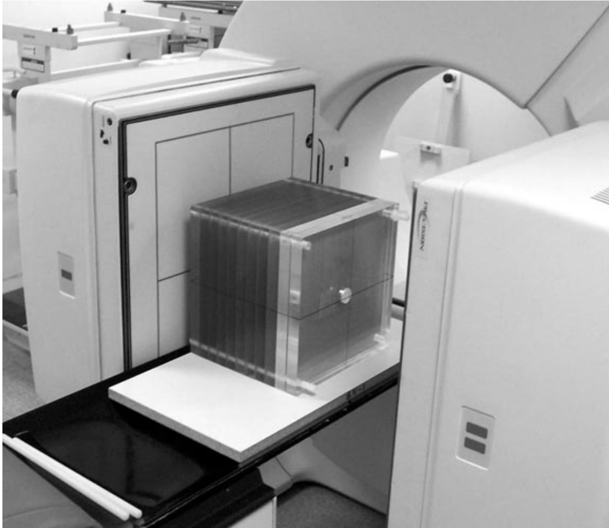
Figure 1-18. AXIS Camera Showing Source Mounted in Acrylic Phantom
