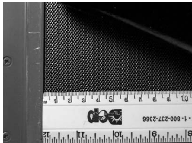
Figure 1-11. Back of Collimator Showing Corrugated Lead Strips
