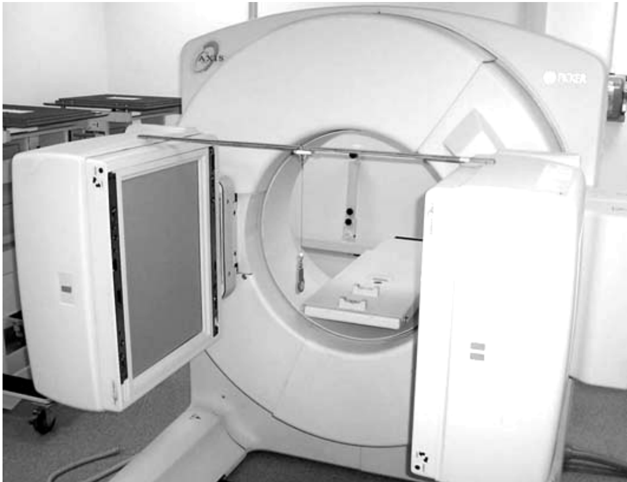
Figure 1-17. AXIS Camera Showing Source Suspended from Meter Stick
