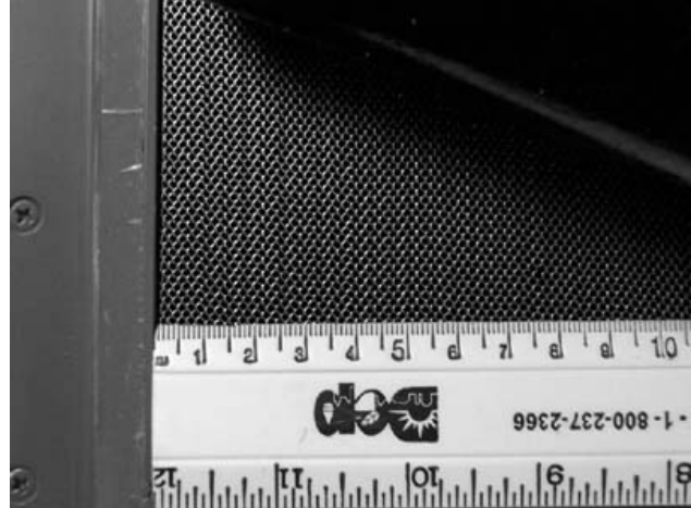
Figure 1-11. Back of Collimator Showing Corrugated Lead Strips
