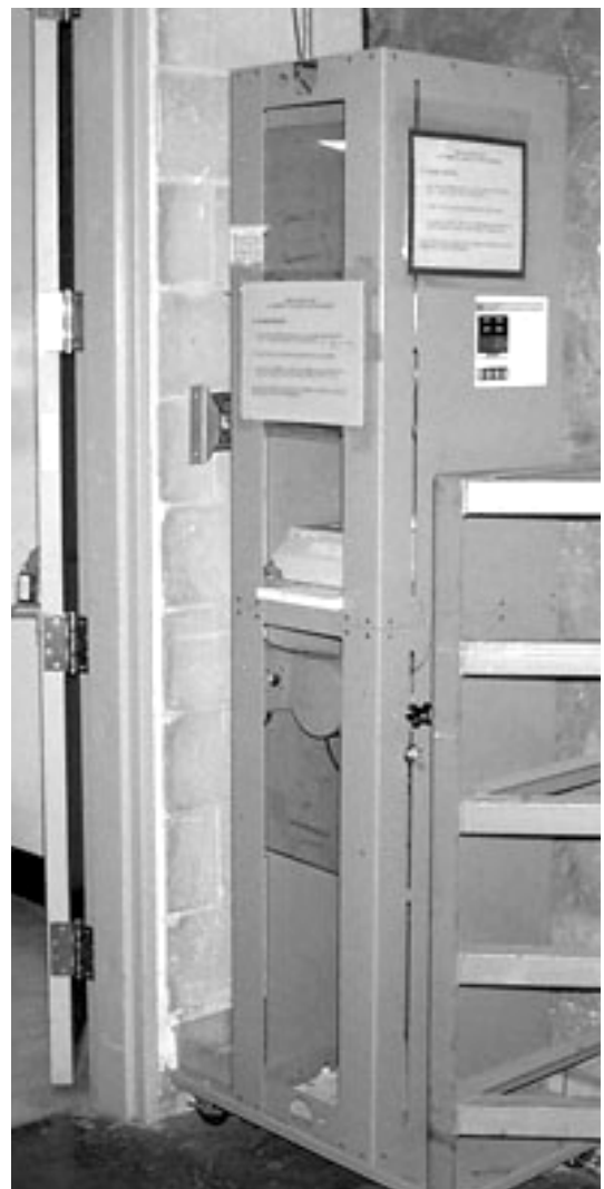
Figure 1-16. Detector Assembly of the HMC Waste Monitor
