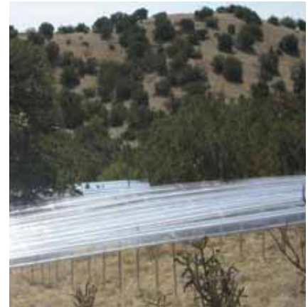
Gutters are used to simulate rainfall scenarios at a study plot.
