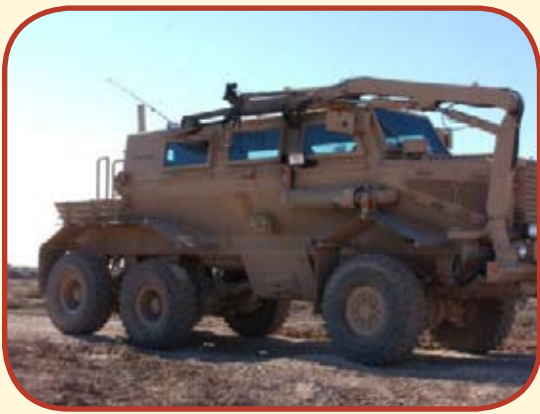
The heavily-armored Buffalo is designed for route clearance, giving patrols a closer look at suspected improvised explosive devices.
