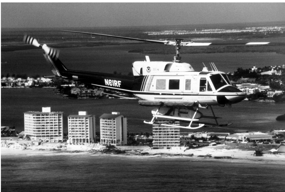
▲ Figure 3. A NOAA Bell helicopter conducts a shallow water survey using the new SHOALS system.
