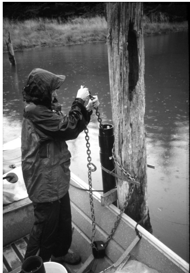
▲ Figure 6. A SWMP technician removing the YSI6000 from the ABS pipe that is attached to the log piling in the bay.
