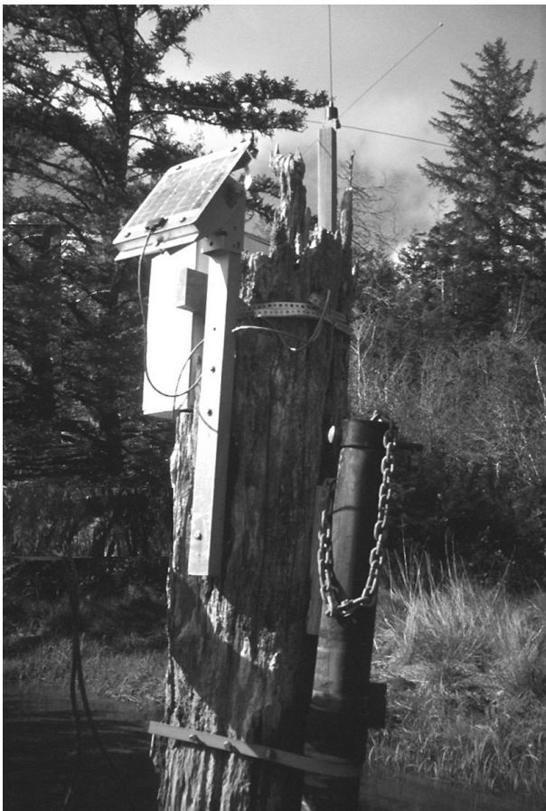
▲ Figure 5. A labeled sonde on site; shows the Winchester SWMP station with a telemetry device attached to transmit real-time data to the interpretive center, for use in a water quality exhibit.
