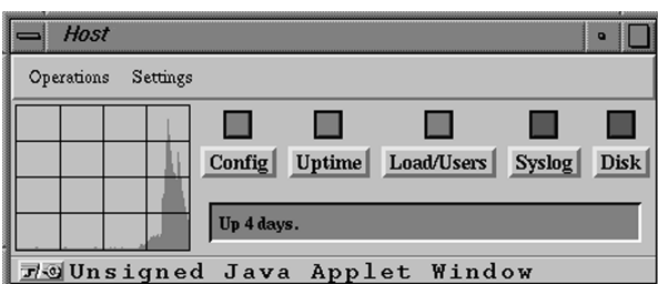
▲ Figure 3. Host status window, which displays alert conditions for a given workstations.
