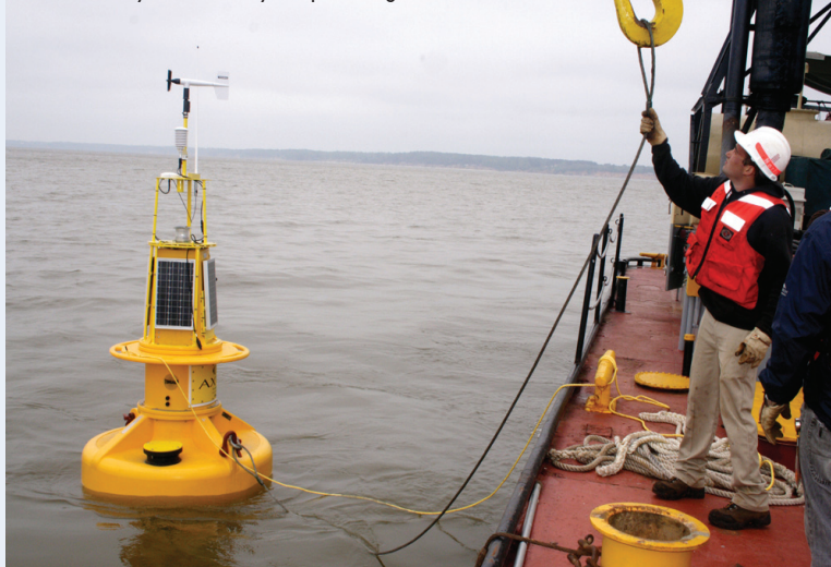
▲ Buoy in the Captain John Smith Chesapeake Water Trail being deployed off shore from a statue of its namesake in Jamestown, Virginia.
