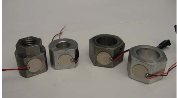
Figure 5: Examples of nuts and washers equipped with PZT wafers.
